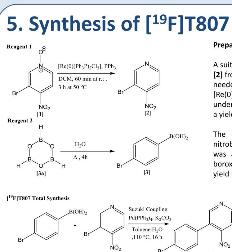
Suzuki Coupling  $Pd(PPh_3)_4, K_2CO_3$ [<sup>19</sup>F]T807 Toluene:H<sub>2</sub>O .110 °C. 16 h
